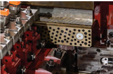
◆ Main Slide Shim-Plated with Self-Lubricant Graphite
